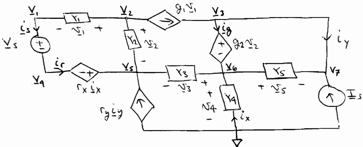
We formulate enough equations to solve for the 7 nodal voltages and the 5 auxiliary currents (2 controlling currents:  $i_x$ ,  $i_y$  and 3 introduced auxiliary currents across voltage sources:  $i_s$ ,  $i_r$ ,  $i_g$ )
