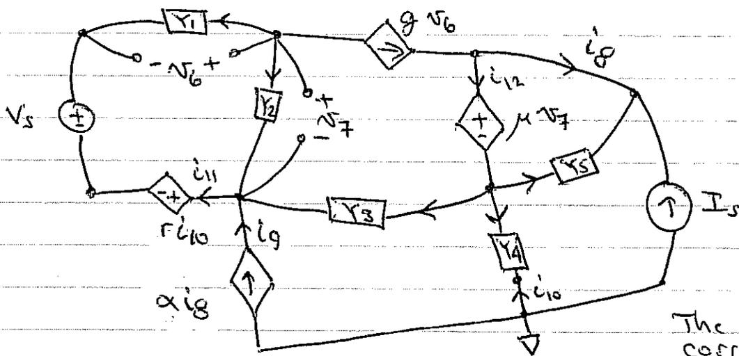
Note that  $i_{10}$  was added on one side of CVT  $V_6$  as one side of VCT and  $V_7$  as one side of VVT.
